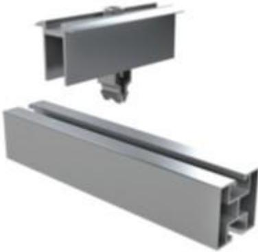
The End and Mid clamps are substantial fully preassembled parts which simply clip into the channel in the rail, and the motion of tightening the screw from the top also fully locks the clamp in place. These substantial mid and End clamps are designed for use for both portrait and landscape installations with the rail installed horizontally.
